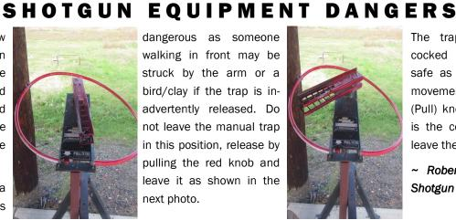
dangerous as someone walking in front may be struck by the arm or a bird/clay if the trap is inadvertently released. Do not leave the manual trap in this position, release by pulling the red knob and leave it as shown in the next photo.
