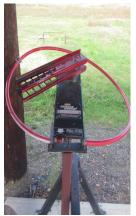
The trap is in the 3/4 cocked position: this is safe as there will be no movement if the release (Pull) knob is pulled. This is the correct position to leave the manual trap.
